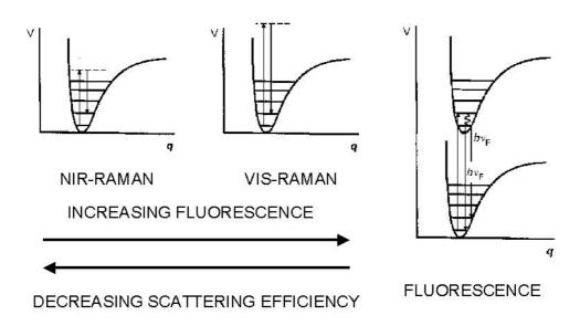
Figure 5. Fluorescence and scattering efficiency in NIR- and VIS-Raman spectroscopy.
