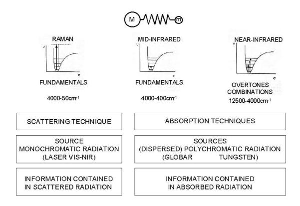
Figure 1. Characteristic vibrational transitions, wavenumber regions and principal physical differences between MIR, NIR and Raman spectroscopy.
