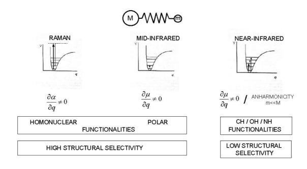
Figure 2. Excitation conditions and structural specificities of the different vibrational spectroscopic techniques.
