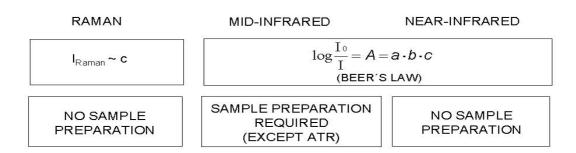
Figure 3. Quantitative and sample preparation aspects of Raman, mid-infrared and near-infrared spectroscopy.
